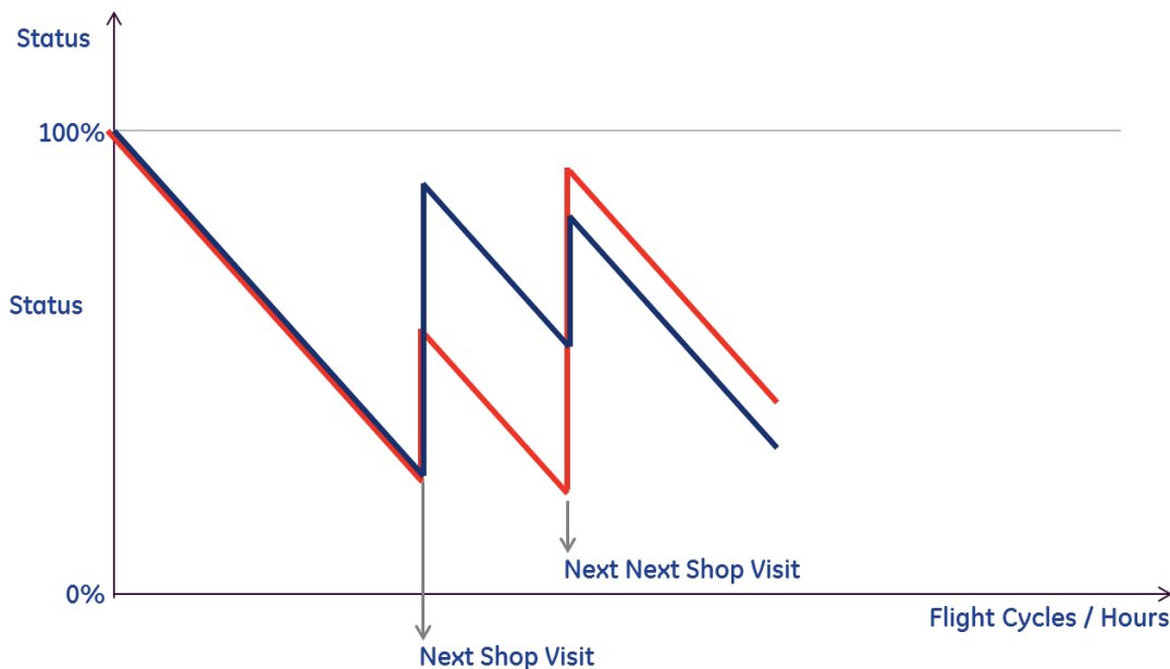
Figure 16: The first limiter will determine the time for the first shop visit of an engine. It is then a matter of optimization how to build up the engine for the second and third intervals.
